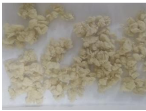
1.rasm. Paxta lintining oqartirishdan oldin(a) va keyingi(b) holati
