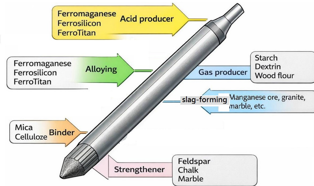
Figure 1. Electrode components and their functions
