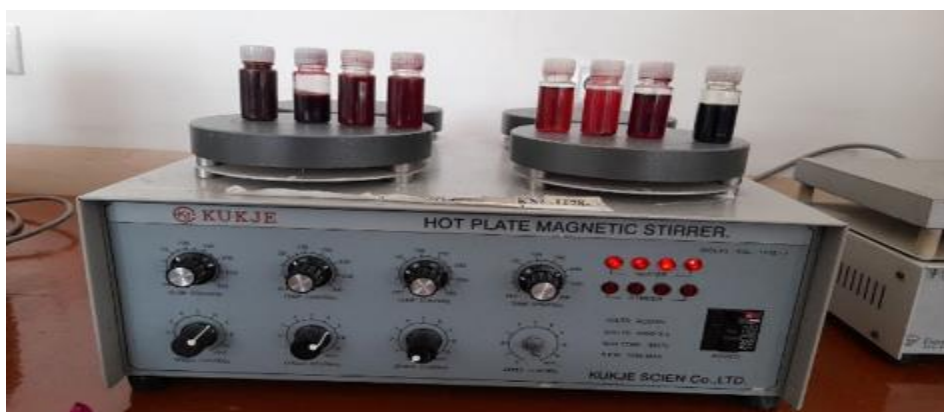
Figure 3 The process of mixing the paint mixture.
